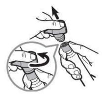
STEP TWO: Bulb located in the bottom portion of otoscope head (see arrow)
